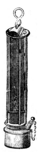
When this lamp is immersed in an explosive mixture of marsh-gas or coal-gas and common air, the gauze cylinder becomes filled with a blue flame, arising from the combustion of the gas within; but the flame does not communicate to the outside, even though the gauze may be heated to less redness.
